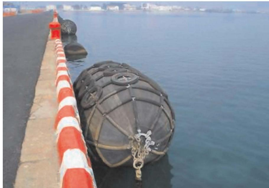
Pneumatic fender is a leading anti-collision device for marine applications in the world today. This fender is made of synthetic-cord-reinforced rubber sheets with compressed air inside to enable it to float on the water and work as a protective medium. Therefore, pneumatic rubber fenders serve as a critical protective medium against collision when ship-to-ship (STS) transfer operations and ship-to-dock (STD) berthing and mooring operations.
